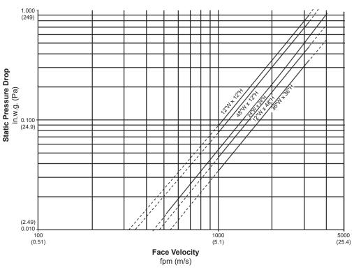
Tested in accordance with AMCA Standard 500D, Figure 5.3 Intake air converted to standard air density.
