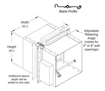
\*Dampers smaller than minimum frame size require a transition. Reference SD-TRFS. Dampers less than 6"H will have a 20" sleeve with the additional sleeve length on the jackshaft side when a B-Pan type transition is ordered.
