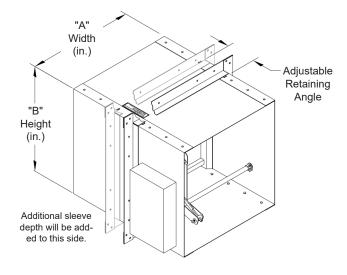
\*Dampers smaller than minimum frame size require a transition. Reference SD-TRFS. Dampers less than 6"H will have a 20" sleeve with the additional sleeve length on the jackshaft side when a B-Pan type transition is ordered.
