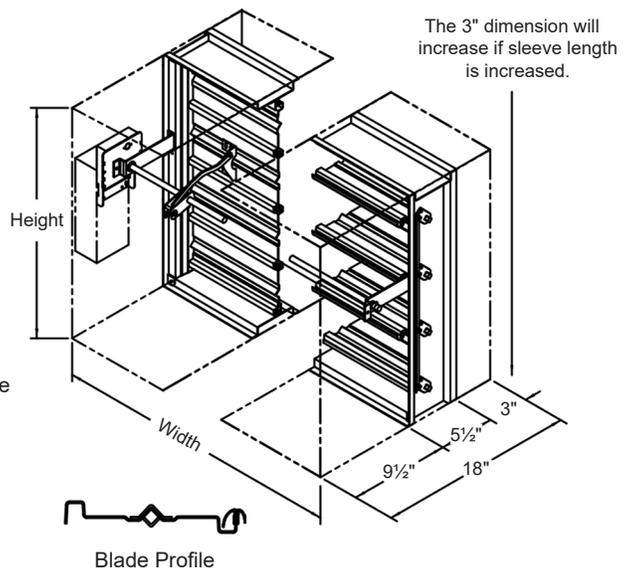
Combination Fire/Smoke Damper • 1½ Hr. Rated • Single Thickness Blade • Leakage Class I • 250°F or 350°F Rated • Galvanized Steel
