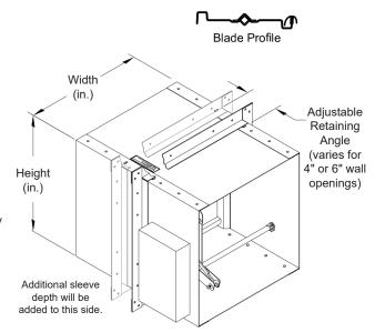
\*Dampers smaller than minimum frame size require a transition. Reference SD-TRFS. Dampers less than 6"H will have a 20" sleeve with the additional sleeve length on the jackshaft side when a B-Pan type transition is ordered.
