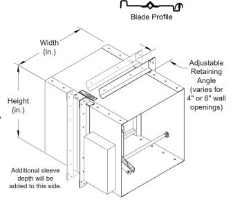
Combination Mini-Fire/Smoke Damper • 11/2 Hour Rated • Leakage Class I • Single Thickness Blade • Integrated Sleeve • 250°F or 350°F Rated • Galvanized Steel
