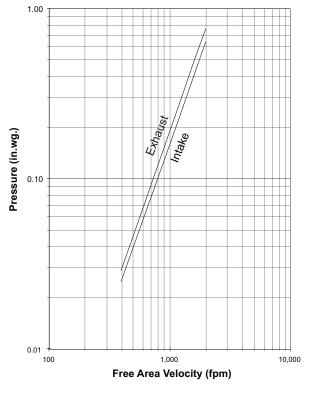
Louver Test Size = 48" x 48" (1219 x 1219) Pressure loss tested in accordance with Figure 5.5 of AMCA Standard 500-L. Data corrected to standard air density.
