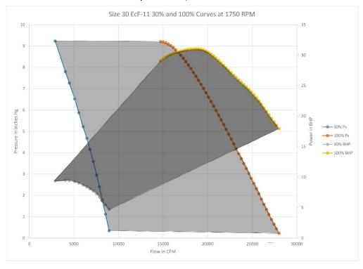
Performance certified is installation Type A: Free inlet, free outlet. Power rating (BHP) does not include transmission losses. Performance ratings do not include the effects of appurtenances (accessories).
