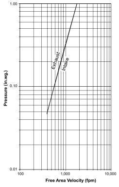
Louver Test Size =  $48" \times 48"$  (1219  $\times$  1219) Pressure loss tested in accordance with Figure 5.5 of AMCA Standard 500-L. Data corrected to standard air density.
