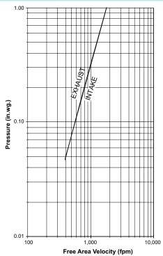
Louver Test Size = 48" x 48" (1219 x 1219) Pressure loss tested in accordance with Figure 5.5 of AMCA Standard 500-L. Data corrected to standard air density.
