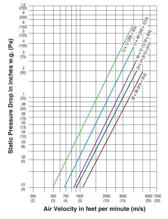
Pressure drop tested per AMCA Standard 500-D, Figure 5.3. Data corrected to standard air density of 0.075 lbs/ft.3.
