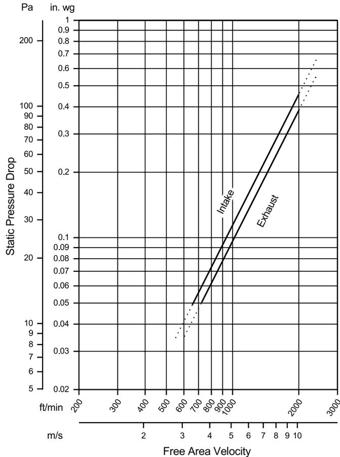
Model K8206A resistance to airflow (pressure drop) varies depending on louver application (air intake or air exhaust). Free area velocities (shown) are higher than average velocity through the overall louver size. See louver selection information. (Test Figure 5.5-6.5)
