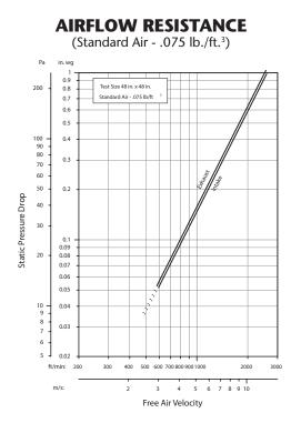
Louver Type T6786 resistance to airflow is shown with louver blades fully open. Resistance (pressure drop) varies depending on louver application (air intake or air exhaust). Free area velocities (shown) are higher than average velocity through the overall louver size (Test Figure 5.5).
