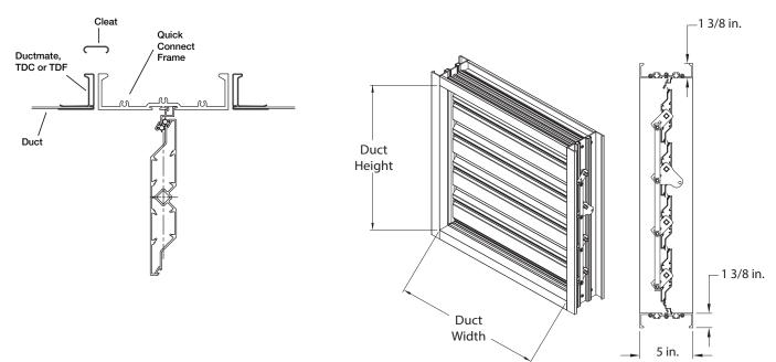
**Note:** When ordering the Quick Connect Frame, size is based on duct size (or inside dimension of the damper frame). Quick Connect frame is actual size.
