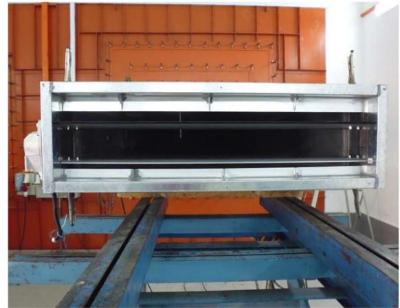
Figure 5.3-6.5 setup Air Performance - Pressure Drop Test
