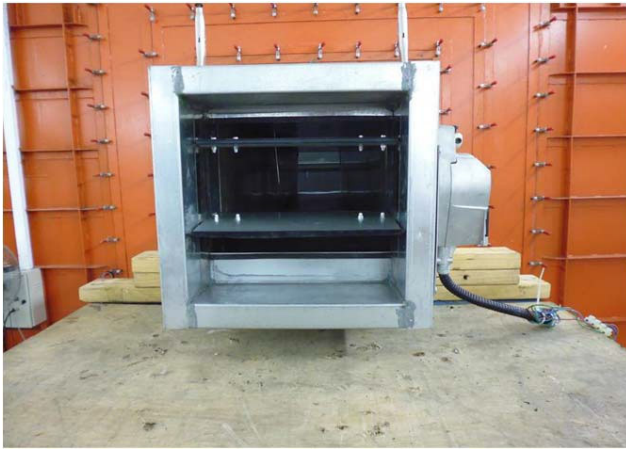
Figure 5.3-6.5 setup Air Performance - Pressure Drop Test
