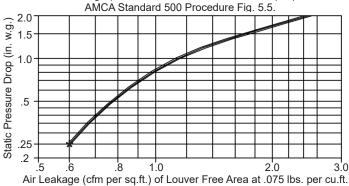
\*Intake air converted to standard air density. Tested to AMCA Standard 500-L, Figure 5.5.
