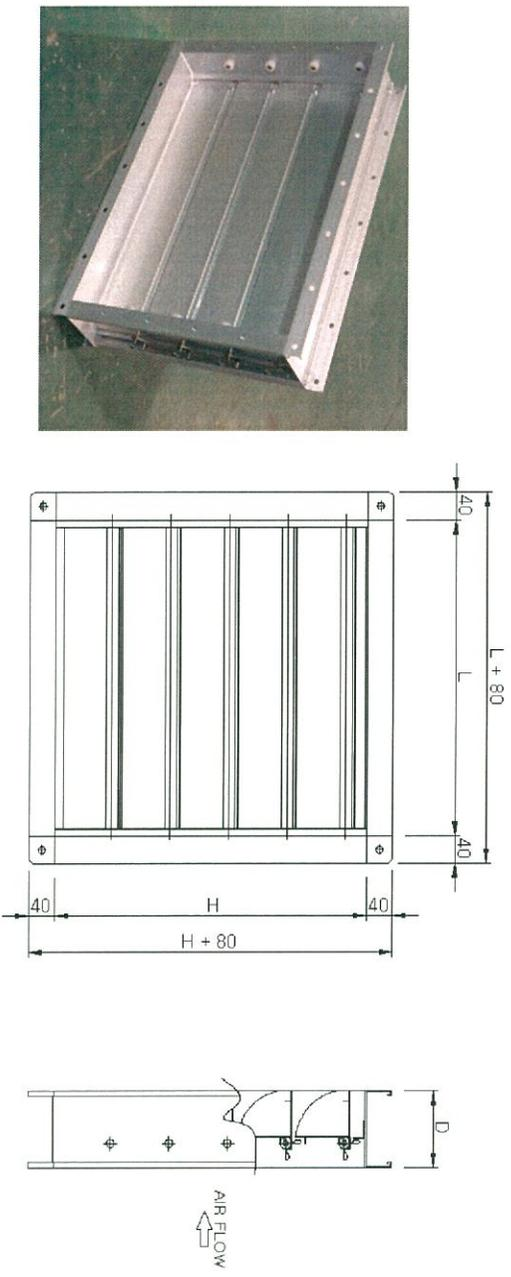
CHECK DAMPERS ARE USED WHERE BACK DRAFT AIR FLOW SHOULD BE SEALED. THE PARALLEL BLADES ARE AUTOMATICALLY OPERATED BY POSITIVE AIR PRESSURE WITH NO NEED TO HAVE A SEPARATE ACTUATOR, FREE OF MAINTENANCE. THE LIGHT AND STURDY ALUMINIUM ENABLES THE DAMPERS TO OPERATE BETWEEN 10mmAq TO 150mmAq.
