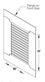
Four-Sided Flange Internal Mount (single section only) \*Grille dimensions furnished approximately 1/2" (13) undersize
