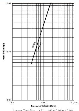
$\begin{array}{l} \mbox{Louver Test Size} = 48" \times 48" \mbox{(}1219 \times 1219\mbox{)} \\ \mbox{Pressure loss tested in accordance with Figure 5.5 of AMCA Standard} \\ \mbox{500-L. Data corrected to standard air density.} \end{array}$
