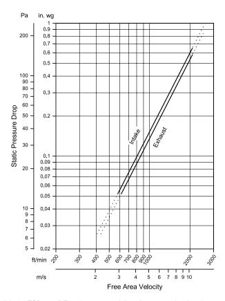
Model ESD-635DE resistance to airflow (pressure drop) varies depending on louver application (air intake or air exhaust). Free area velocities (shown) are higher than average velocity through the overall louver size. See louver selection information. (Test Figure 5.5-6.5)
