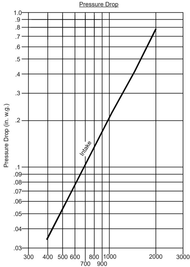
Intake air converted to standard air density.
