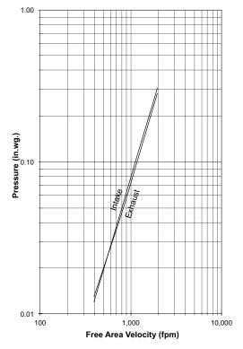
Louver Test Size = 48" x 48" (1219 x 1219) Pressure loss tested in accordance with Figure 5.5 of AMCA Standard 500-L. Data corrected to standard air density.
