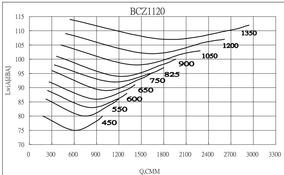
**Sound Power [dB Ref 10-12 watts] %POF=( CMM\*3531.5 / RPM x 82.32 )**
