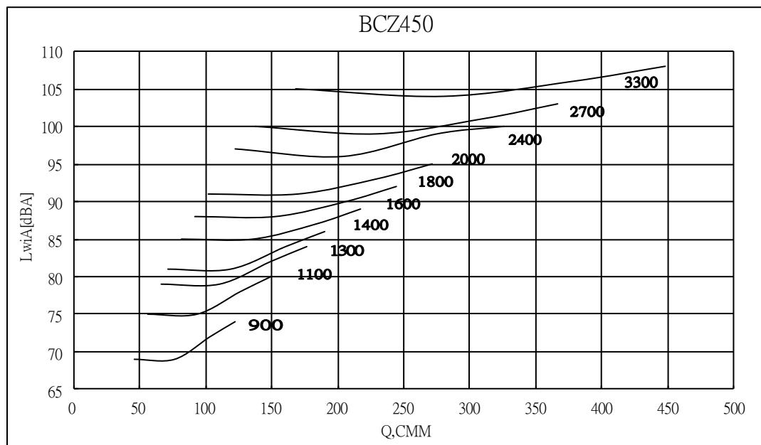
**Sound Power [dB Ref 10-12 watts] Inlet Sound Power, Lwi [ Octave Band ]**
