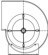
**Type L** This type is supplied with mounting feet and can be mounted in three different orientations. Inlet flange 'L' and outlet flange are supplied as standard.
