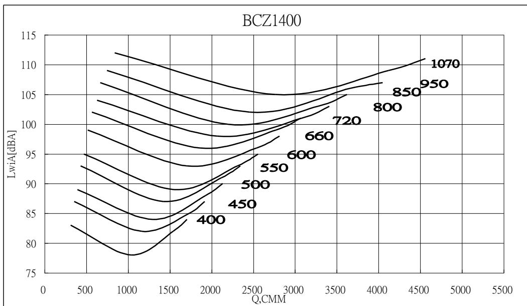
**Sound Power [dB Ref 10-12 watts] %POF=( CMM\*3531.5 / RPM x 160.77 )**
