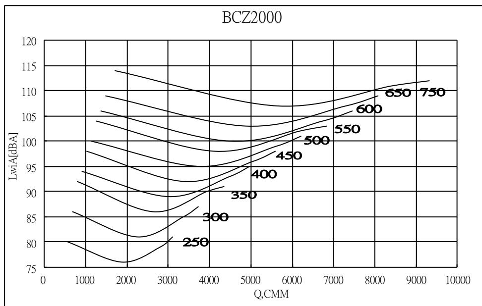
**Sound Power [dB Ref 10-12 watts]    %POF=( CMM\*3531.5 / RPM x 468.73 )**
