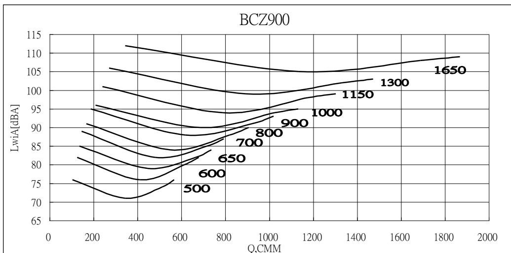
**Sound Power [dB Ref 10-12 watts]    Inlet Sound Power, Lwi [ Octave Band ]**
