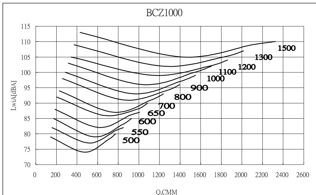
**Sound Power [dB Ref 10-12 watts] %POF=( CMM\*3531.5 / RPM x 58.59 )**
