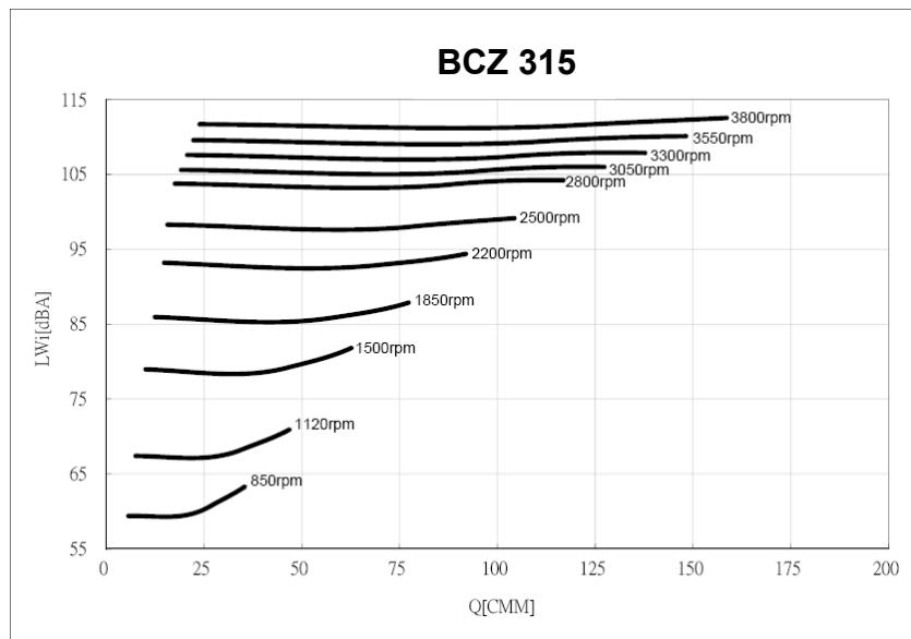
**Sound Power [dB Ref 10-12 watts] %POF=( CMM\*3531.5 / RPM x1.47 )****Inlet Sound Power, Lwi [ Octave Band ]**
