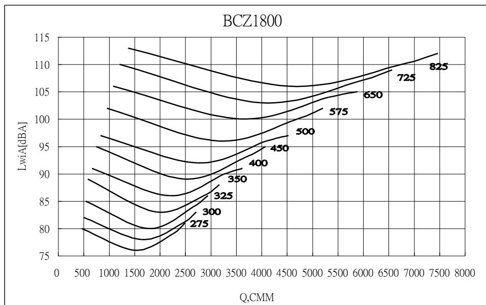
**Sound Power [dB Ref 10-12 watts] %POF=( CMM\*3531.5 / RPM x 341.7 )**
