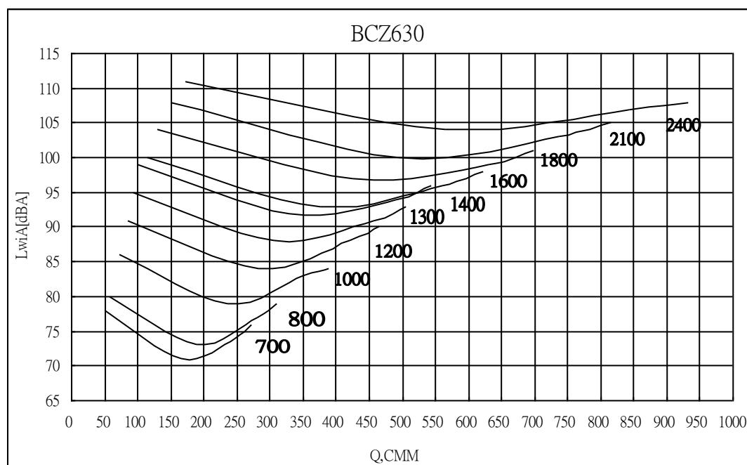
**Sound Power [dB Ref 10-12 watts]    Inlet Sound Power, Lwi [ Octave Band ]**
