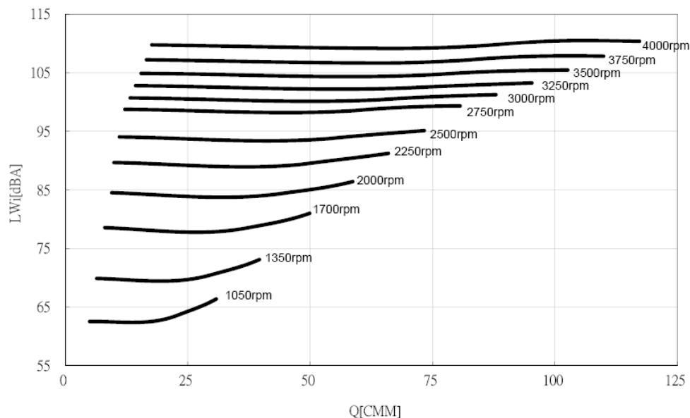
**Sound Power [dB Ref 10-12 watts] %POF=( CMM\*3531.5 / RPM x 1.03 )**
