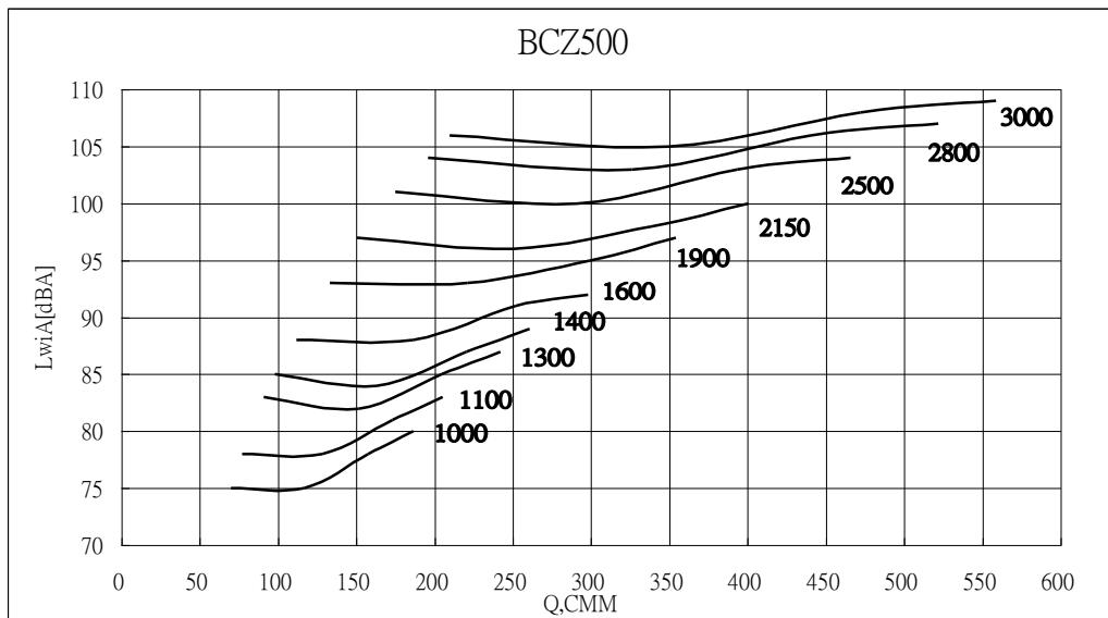
**Sound Power [dB Ref 10-12 watts]    Inlet Sound Power, Lwi [ Octave Band ]**
