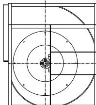
**Type V** This type is similar to type H but utilizes enhanced bearings to support higher load necessary for the increased performance.
