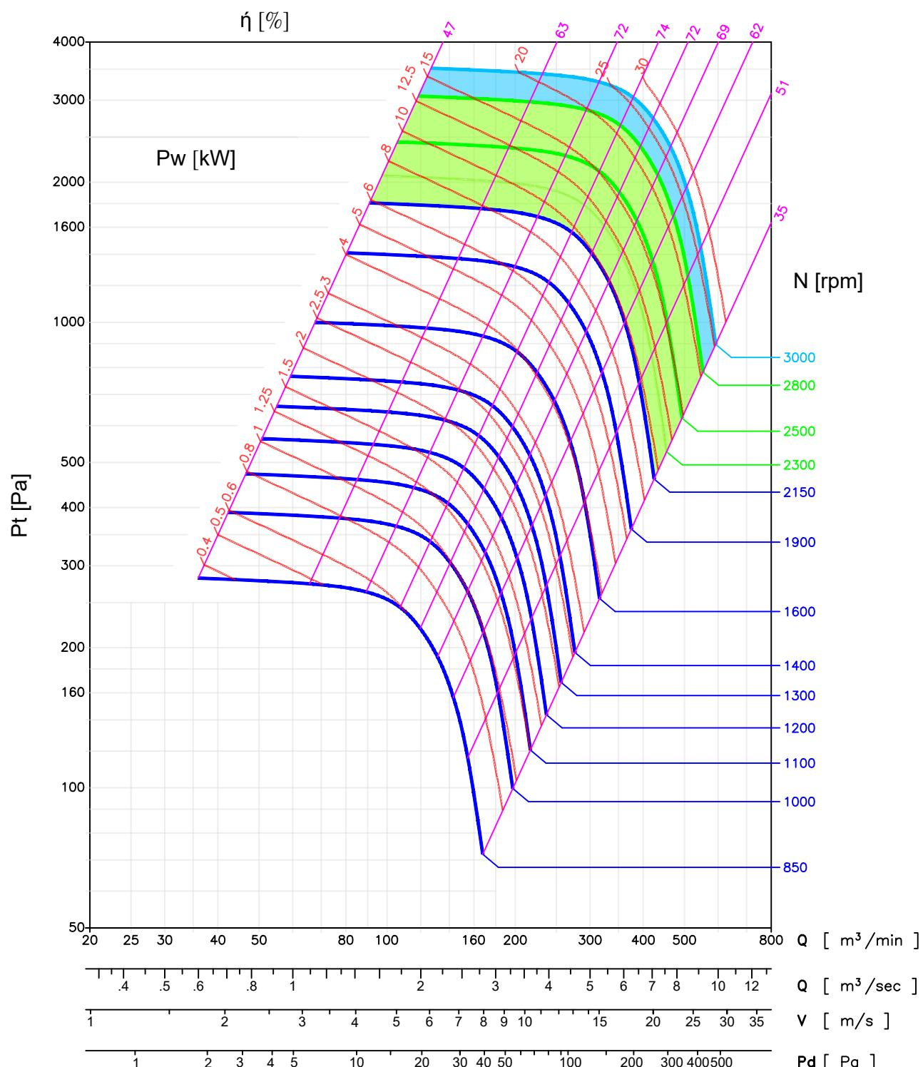
— Performance certified is for installation type B – free inlet, ducted outlet. Performance ratings do not include the effects of appurtenances(accessories). Power rating (kW) does not include transmission losses.
