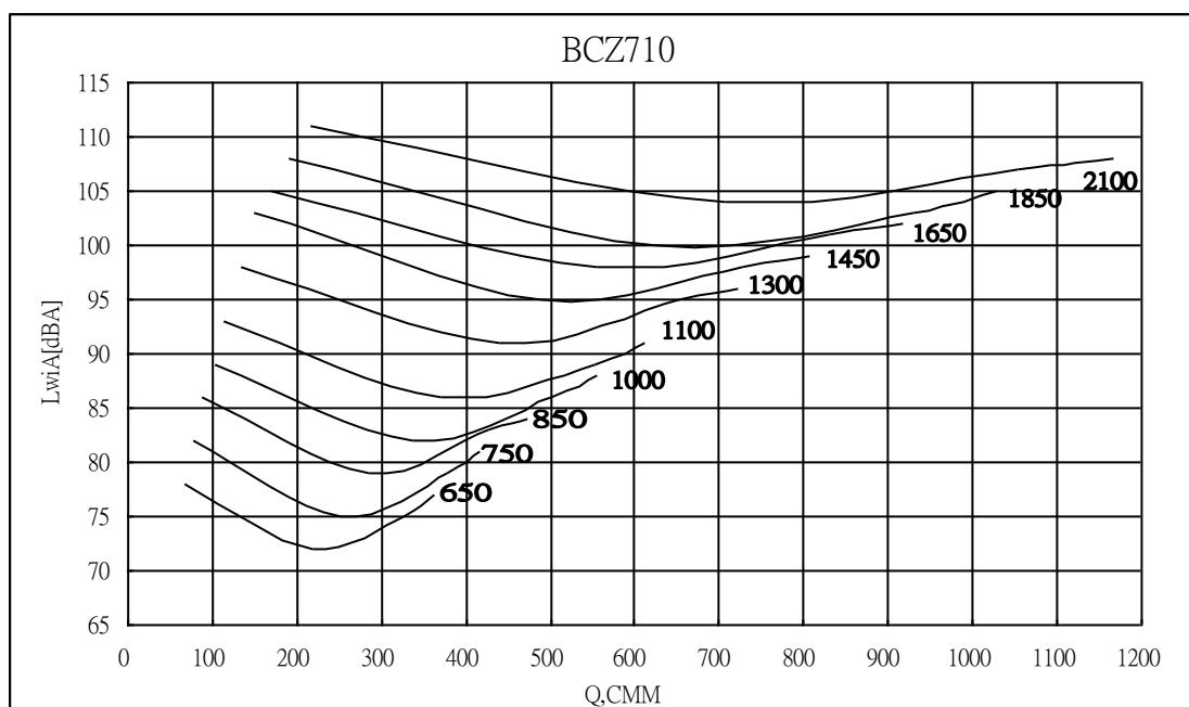
**Sound Power [dB Ref 10<sup>-12</sup> watts] Inlet Sound Power, Lwi [ Octave Band ]**
