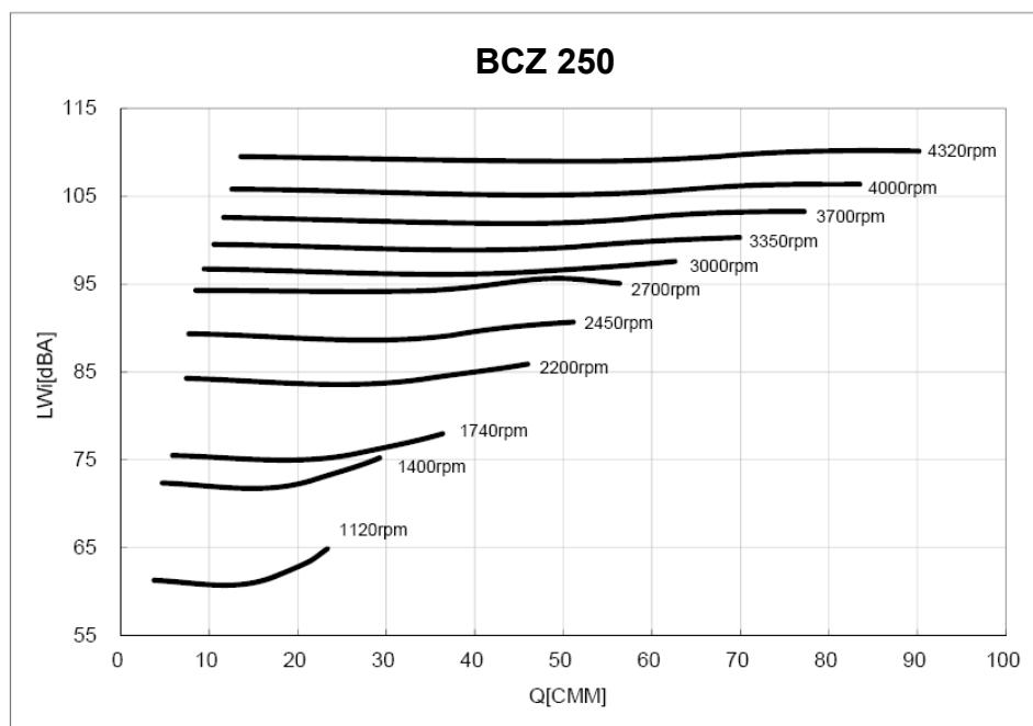
**Sound Power [dB Ref 10-12 watts] %POF=( CMM\*3531.5 / RPM x 0.74 )**
