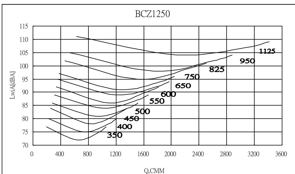
**Sound Power [dB Ref 10-12 watts] %POF=( CMM\*3531.5 / RPM x 114.44 )**
