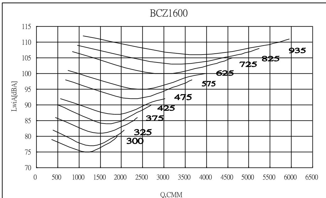
**Sound Power [dB Ref 10-12 watts] %POF=( CMM\*3531.5 / RPM x 239.99 )**
