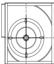
**Type M** This type has a frame fitted on both sides of the fan which gives better strength and rigidity and allows mounting in four different orientations.
