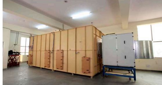
Blowtech's Fan Test Lab as per AMCA210
