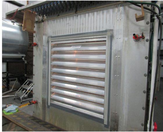
AMCA Standard 500-L-07 Water Penetration Test Test Figure 5.6
