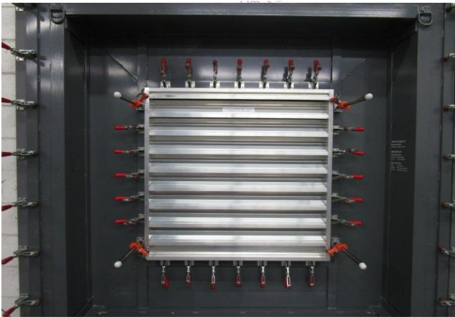
ANSI/AMCA Standard 500-L (Exhaust) Pressure Drop Test Test Figure 5.5
