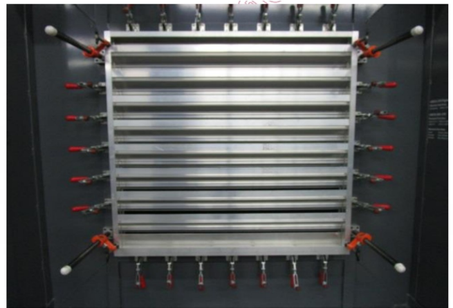
ANSI/AMCA Standard 500-L-12 (Intake) Pressure Drop Test Test Figure 5.5
