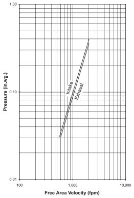
Louver Test Size = 48" x 48" (1219 x 1219) Pressure loss tested in accordance with Figure 5.5 of AMCA Standard 500-L. Data corrected to standard air density.
