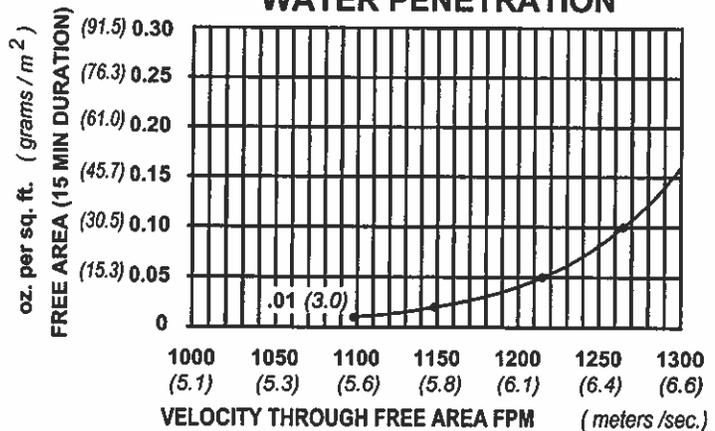
Both maximum recommended free area velocity and beginning of water penetration are 1098 fpm at standard air - .075 lbs. per cu. ft. The above water penetration data is based on mill finish, 48" x 48" test size per AMCA Standard 511.
