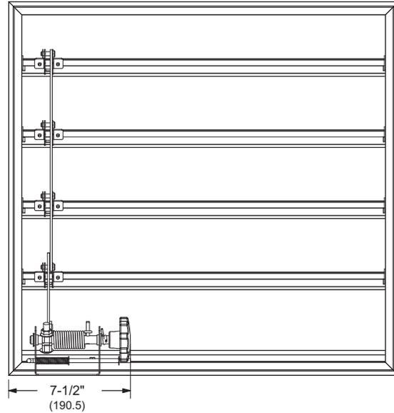
**NOTE:** Adjustable Pressure Controller available on sizes larger than 8.75" x 10.75" (222 x 273) Nominal, 8.5" x 10.5" (216 x 267) Net OD. Adjustable Pressure Controller can be set to maintain a maximum pressure of 0.4 in.wg. (0.01 kPa) for a damper area of 4.0 ft<sup>2</sup> (0.37 m<sup>2</sup>).
