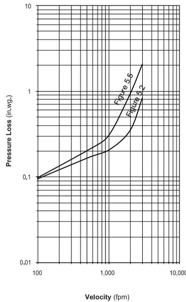
Pressure drop testing was performed in accordance with AMCA Standard 500-D using the two configurations shown. All data has been corrected to represent air density of 0.075 lb/ft. Actual pressure drop in any ducted HVAC system is a combination of many elements. This information, along with analysis of other system influences, should be used to estimate actual pressure losses for a damper installed in a given HVAC system.
