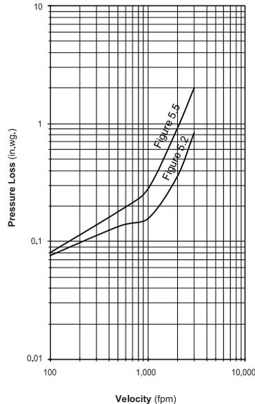
Pressure drop testing was performed in accordance with AMCA Standard 500-D using the two configurations shown. All data has been corrected to represent air density of 0.075 lb/ft. Actual pressure drop in any ducted HVAC system is a combination of many elements. This information, along with analysis of other system influences, should be used to estimate actual pressure losses for a damper installed in a given HVAC system.
