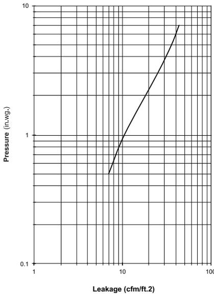
Leakage testing was conducted in accordance with ANSI/AMCA 500-D, Figure 5.5, in the intake direction. Data are based on a vertically mounted damper, with gravity used as the only closing torque. Air leakage is based on operation between 32°F (0°C) and 120°F (49°C) and converted to standard air density.
