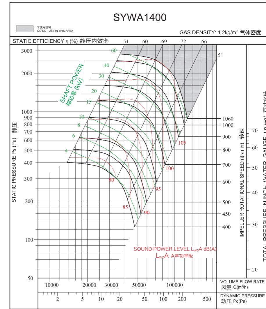
Measured in installation A according to AMCA Standard 210:
