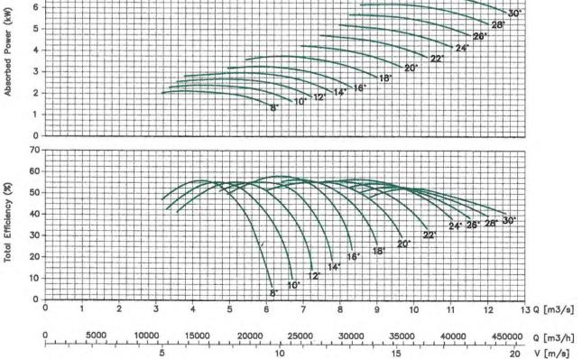
Performance shown is for installation type D - ducted inlet, ducted outlet. Performance ratings do not include the effects of appurtenances in the airstream.
