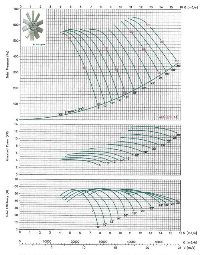
Performance shown is for installation type D - ducted inlet, ducted outlet. Performance ratings do not include the effects of appurtenances in the airstream.
