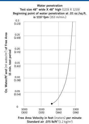
AMCA Standard 500 provides a reasonable basis for testing and rating louvers. Testing to AMCA 500 is performed under a certain set of laboratory conditions. This does not guarantee that other conditions will not occur in the actual environment where louvers must operate.
