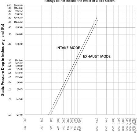
Test size 48" x 48" (1219 x 1219) Ratings do not include the effect of a bird screen.
