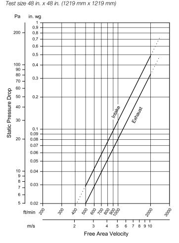
Model EACA-601D resistance to airflow (pressure drop) varies depending on louver application (air intake or air exhaust). Free area velocities (shown) are higher than average velocity through the overall louver size. See louver selection information. (Test Figure 5.5-6.5)
