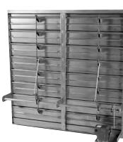
The flanged frame damper is designed to recess inside the flanges of the optional wall housing or wall mounting collar. The center pivot style damper provides superior weather resistance. Galvanized (optional aluminum) construction is rated to 3500 FPM with proper clearance as provided by all factory accessories.
