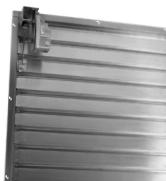
The motorized option improves weather protection by providing a tighter closure seal and is recommended for all supply applications. Heavy-duty dampers are constructed with galvanized frames and blades and are rated to 3000 FPM. The damper body is not recessed providing extra clearance between the fan and damper blades.
