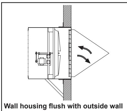
Wall housing flush with outside wall
