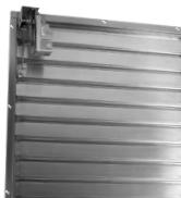
The motorized option improves weather protection by providing a tighter closure seal and is recommended for all supply applications. Standard duty dampers are constructed with galvanized frames and aluminum blades and are rated to 2000 FPM. The damper body is not recessed providing extra clearance between the fan and damper blades.
