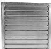
This damper can greatly reduce the infiltration of outside air and although not completely watertight, will provide weather protection in an economical fashion. Constructed with a galvanized frame and aluminum blades this damper is rated to 2000 FPM with the proper clearance as provided by all factory accessories. The damper body is recessed into the opening for a flush appearance.
