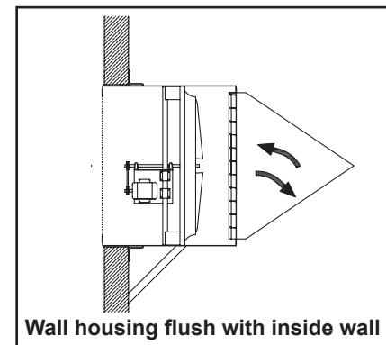
Wall housing flush with inside wall
