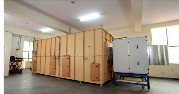
Blowtech's Fan Test Lab as per AMCA210
