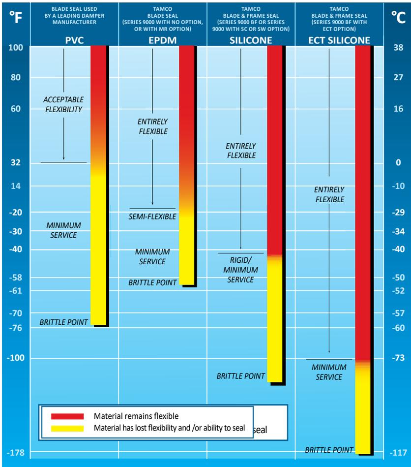
Minimum service temperatures and brittle points are as stated by material manufacturers. Flexibility, rigidity, and suitability status of various materials were determined by observation and operation of dampers in both cold room and cold box environments.
