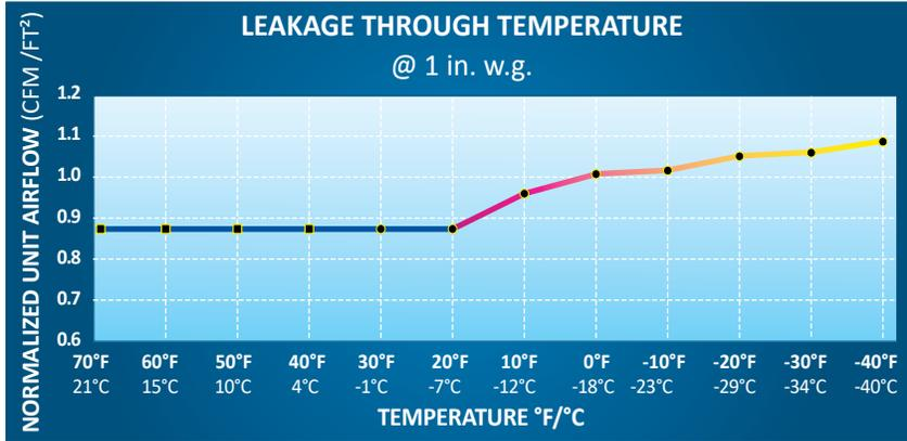
Damper tests were conducted in a laboratory cold room to determine the effects of colder and severe cold temperatures (down to -40°F (-40°C)) on sealing gaskets and leakage rates.
