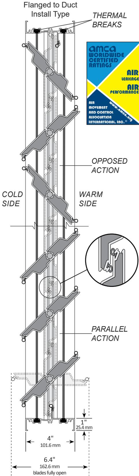
1. Extruded aluminum (6063-T5) damper frame is not less than 0.080" (2.03 mm) in thickness. Damper frame is 4" (101.6 mm) deep x 1" (25.4 mm), with mounting flanges on both sides of frame.
