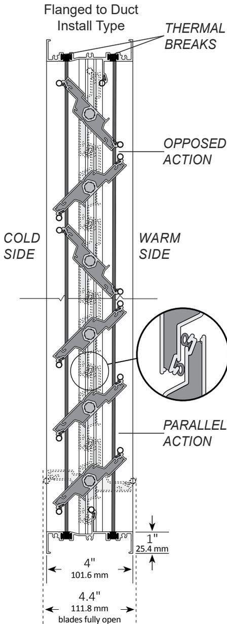
1. Extruded aluminum (6063-T5) damper frame is not less than 0.080" (2.03 mm) in thickness. Damper frame is 4" (101.6 mm) deep x 1" (25.4 mm), with mounting flanges on both sides of frame.
