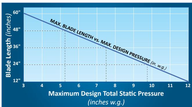
Series 9000 BF dampers, whose blade length exceeds the maximum design pressure, may be reconfigured to maintain a blade length compatible with the required system pressure by increasing the number of sections per damper and thereby reducing each damper section's blade length. Appropriate intermediate structural support will be required for all multiple-section damper assemblies. (Refer to line 14 of the Submittal Data and to TAMCO's Aluminum Damper Installation Guidelines.)
