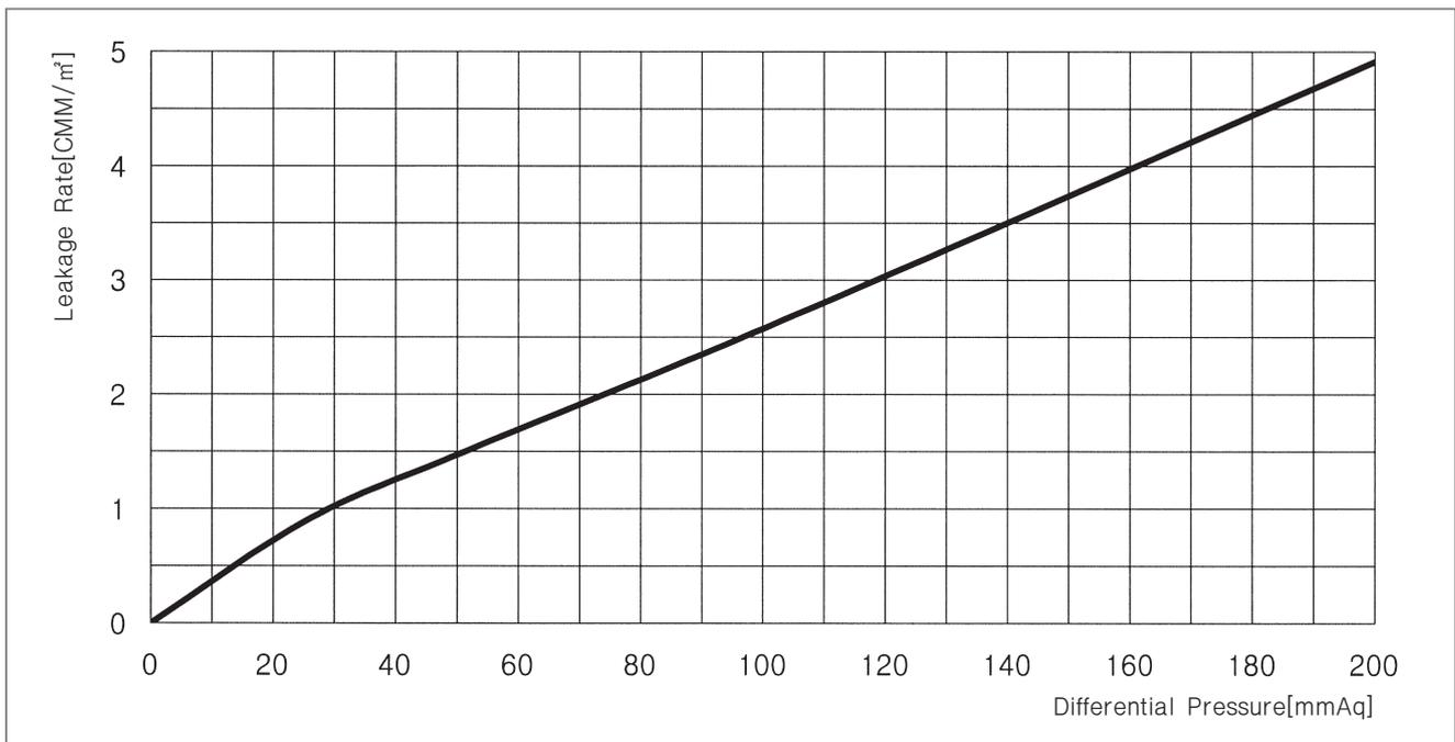
\* Air volumes are based on the density of 1.2Kg/m<sup>3</sup>
