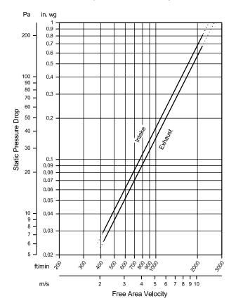
Model K8504 resistance to airflow (pressure drop) varies depending on louver application (air intake or air exhaust). Free area velocities (shown) are higher than average velocity through the overall louver size. See louver selection information. (Test Figure 5.5-6.5)
