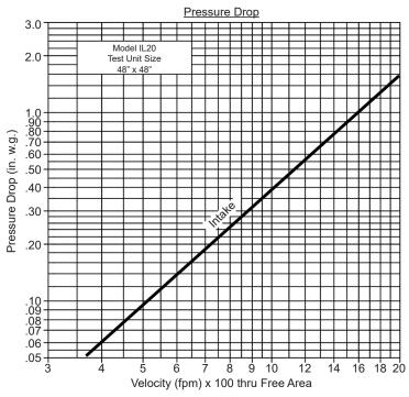
Intake air converted to standard air density.
