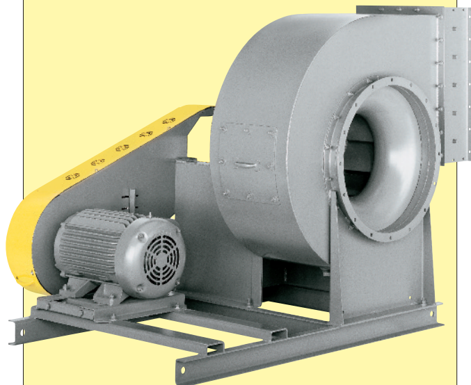
Size 22, Arrangement 1 fan with optional unitary base, flanged inlet and outlet, discharge damper, shaft and bearing guard, belt guard, bolted cleanout door, motor and slide base, and gray epoxy coating.
