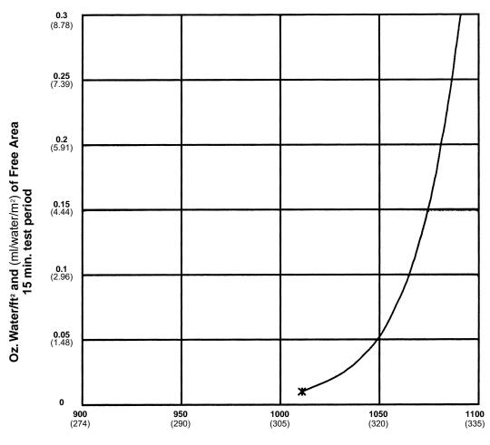
Free Area Velocity in feet and (meters) per minute Standard air .075 lb/ft<sup>3</sup>
