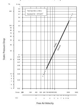
Louver Type K6776 resistance to airflow is shown with louver blades fully open. Resistance (pressure drop) varies depending on louver application (air intake or air exhaust). Free area velocities (shown) are higher than average velocity through the overall louver size. (Tested to Figure 5.5-6.5)
