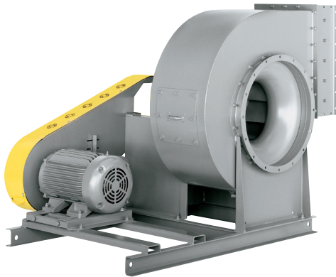
Size 22, Arrangement 1 SWSI fan with optional unitary base, flanged inlet and outlet, outlet damper, shaft and bearing guard, belt guard, bolted cleanout door, motor and slide base, and gray epoxy coating.
